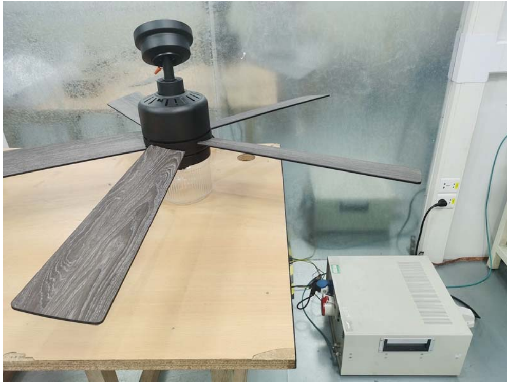
Conducted Emission Test Setup:
