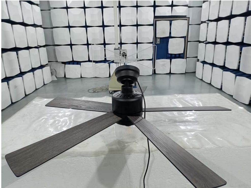
Radiated Emission Test Setup:
