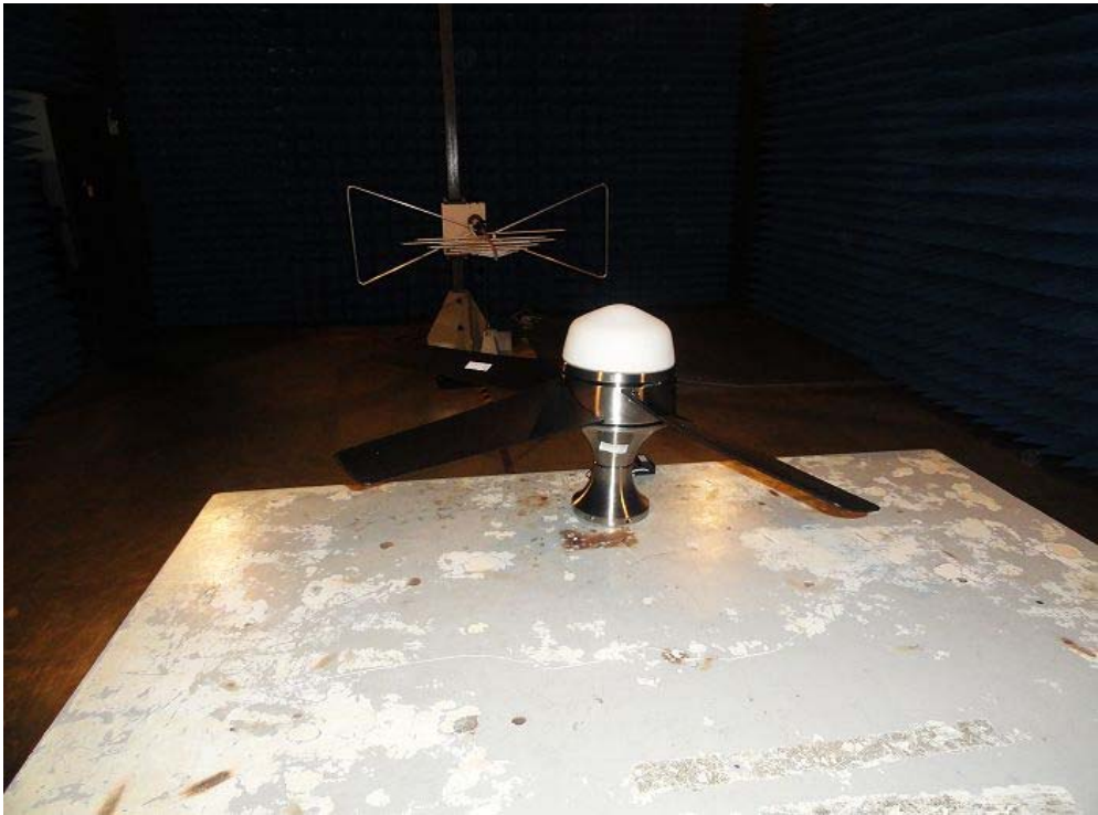
Radiated emission test view--
