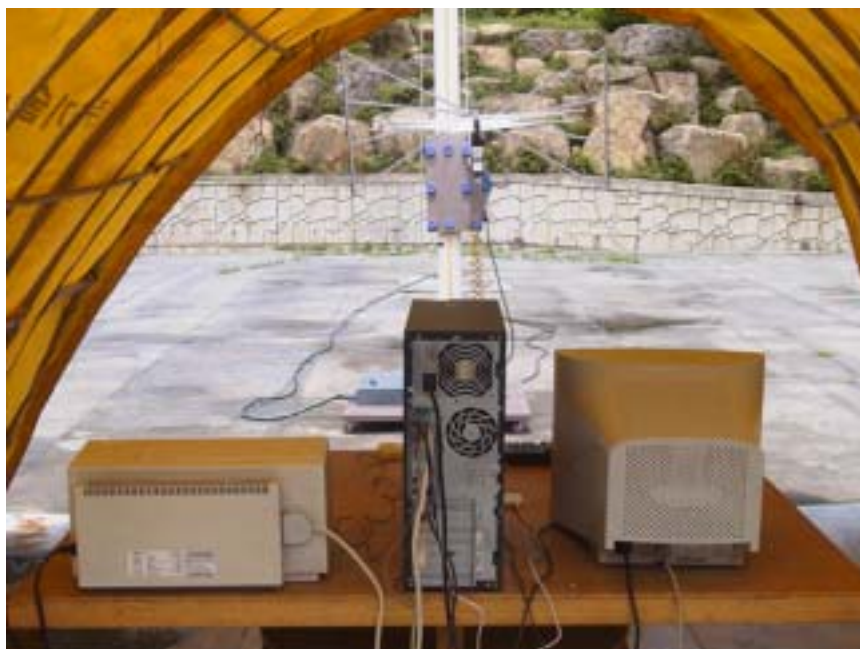
Photograph 1 : Setup for radiated Emissions
