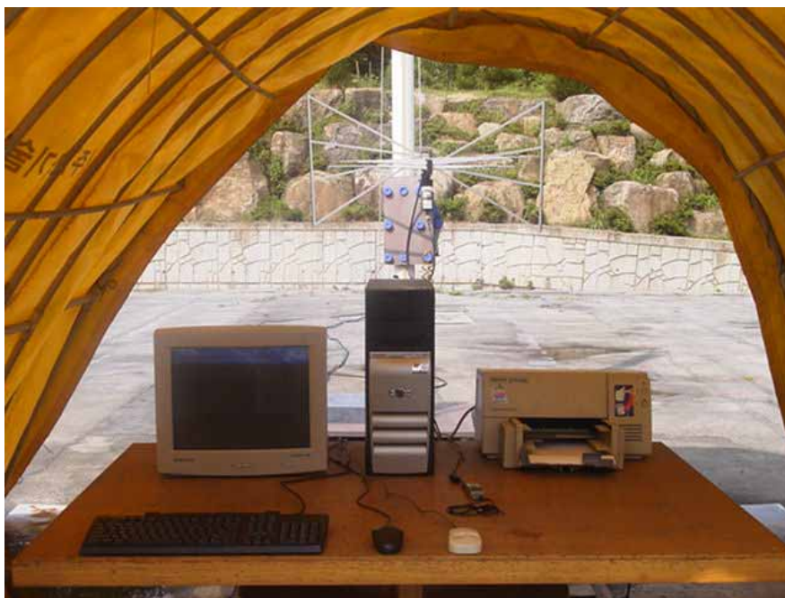
Photograph 1 : Setup for radiated Emissions
