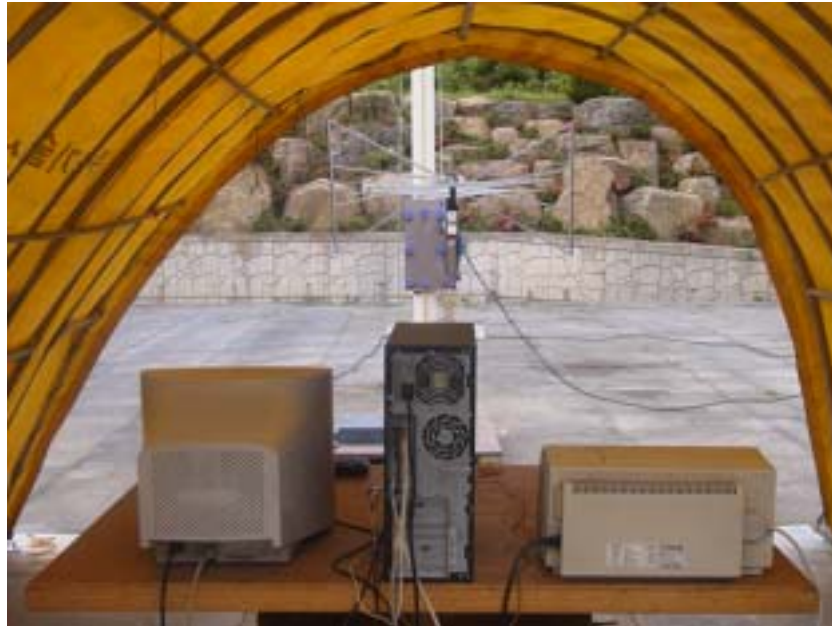
Photograph 1 : Setup for radiated Emissions
