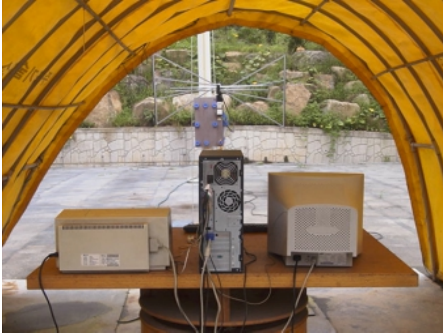
Photograph 1 : Setup for radiated Emissions
