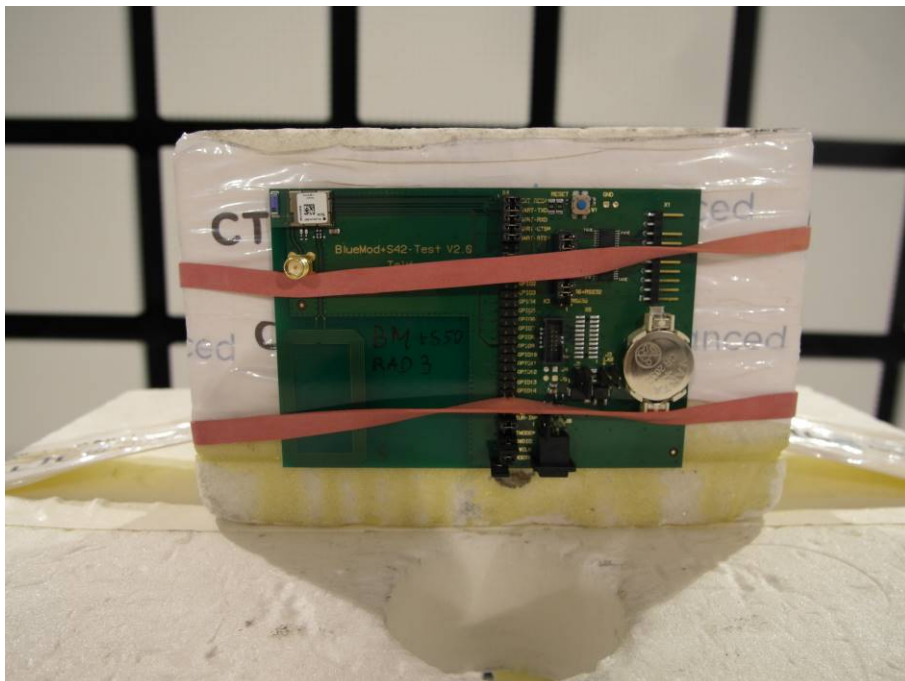
Photo 4: module with on-board antenna
