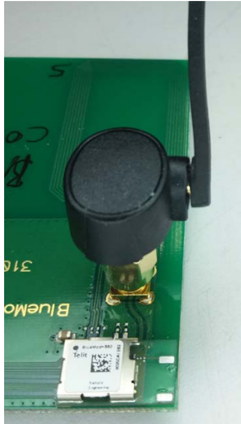
Photo 3: Top view, PMN: BlueMod+S50/AP, soldered to a BlueMod evaluation board.
