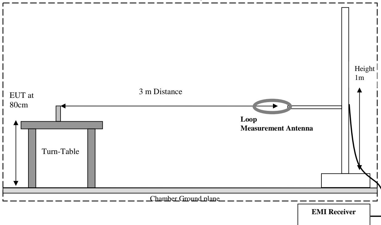
Radiated Emissions Test Setup 30MHz-1GHz Measurements
