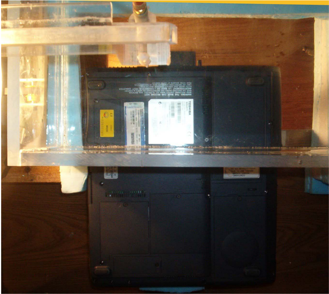
Fig. 2. Photograph of the bottom of the Toshiba Model 1415-S173 Host Computer with RF Micro Devices Cardbus Card Model DK5405 pressed against the bottom of the planar phantom. This is Configuration 1 – Laptop position for SAR testing.
