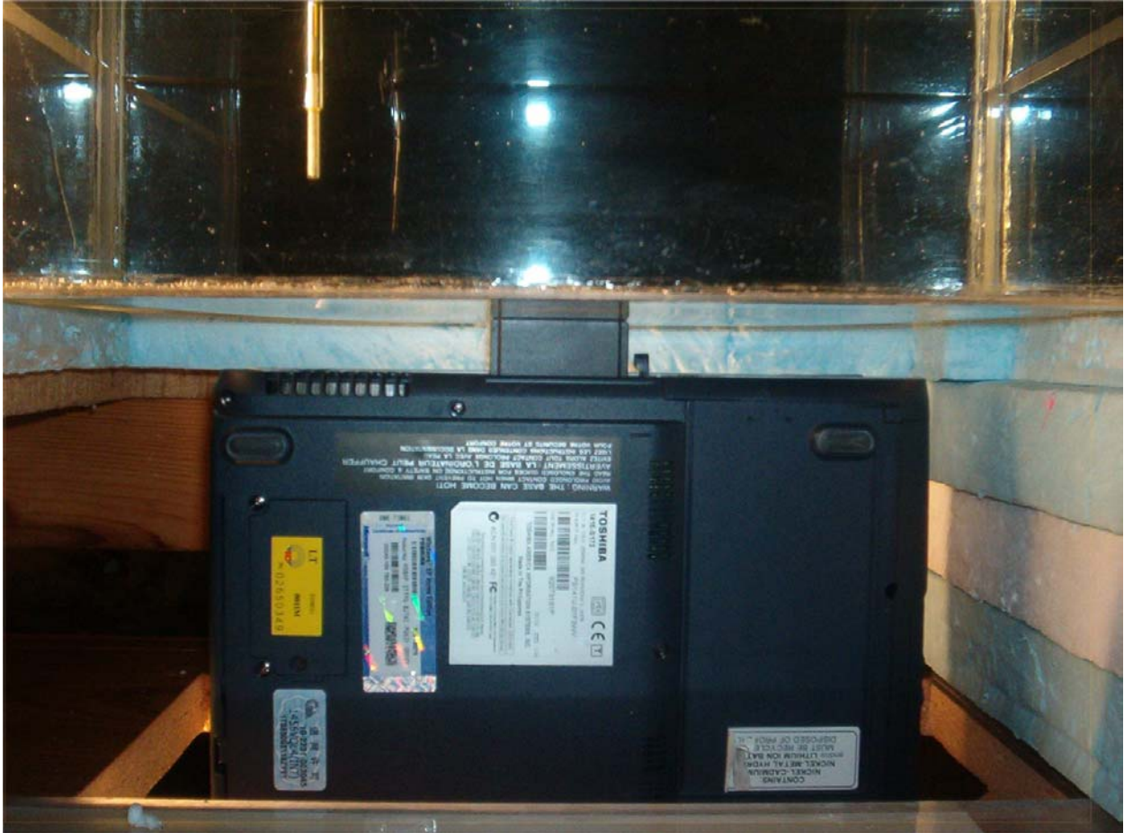
Fig. 3. Photograph of the Toshiba Model 1415-S173 Host Computer at 90° with the edge of the RF Micro Devices Cardbus Card Model DK5405 pressed against the bottom of the planar phantom. This is Configuration 2 for SAR testing and represents the case of a bystander at a distance of 0 cm from the edge of the Cardbus Card.
