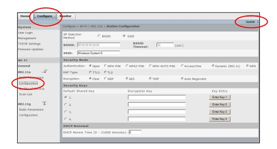
After setting the Station radio parameters, press the "Update" button.
