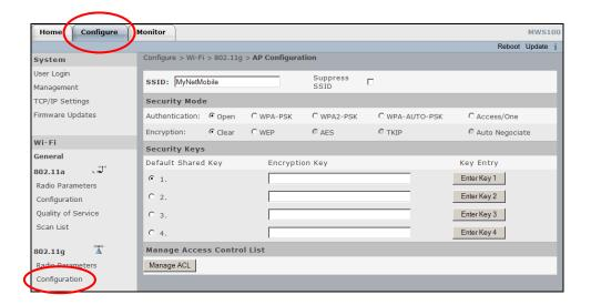
After setting the AP radio parameters, press the "Update" button, then press the "Reboot" button.
