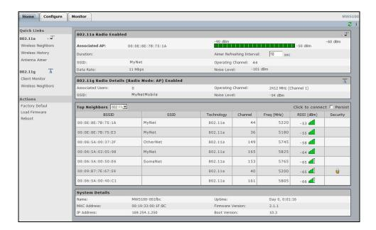
Nearby Wireless Access Points may be viewed on the "Top Neighbors" window of the "Home" screen. This is useful for identifying Strix Access/One® Mesh Nodes that the MWS100 Wireless Station radio may connect to, or for identifying potential sources of interference.
