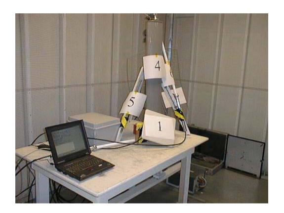
Conducted Emission Test (Front View)
