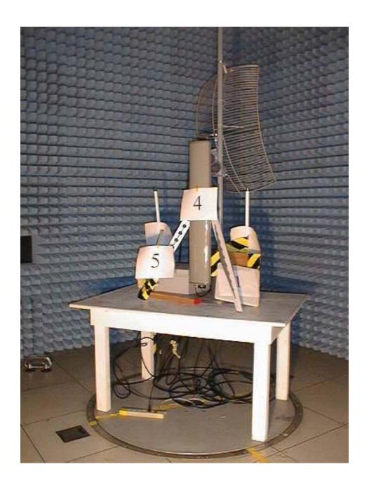
Radiated Emission Test with All Antenna (Front View)
