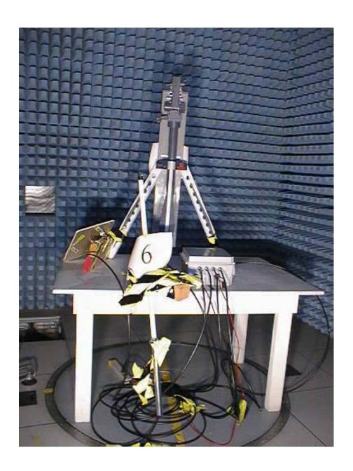
Radiated Emission Test with 4 Antenna (Rear View)
