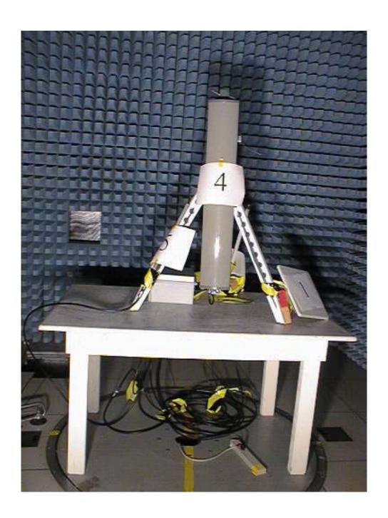
Radiated Emission Test with 4 Antenna (Front View)
