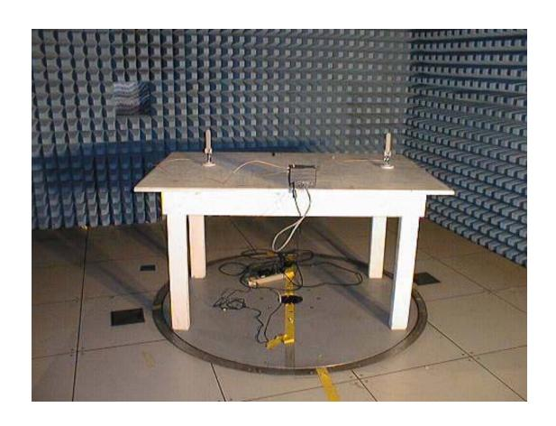
**Radiated Emission Test with External Antenna**
