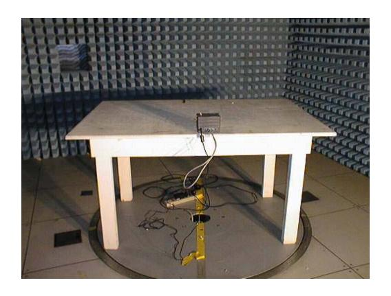
**Radiated Emission Test with Antenna Module**
