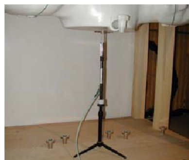
Figure 12.1 Dipole Validation Test Setup
