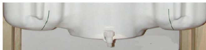
Figure 7.2 SAM Twin Phantom shell
