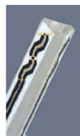
Figure 3.2 Probe Thick-Film Technique
