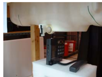
Figure 14.1 Body SAR Test Setup
