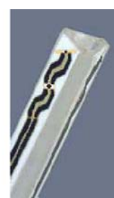
Figure 3.2 Probe Thick-Film Technique
