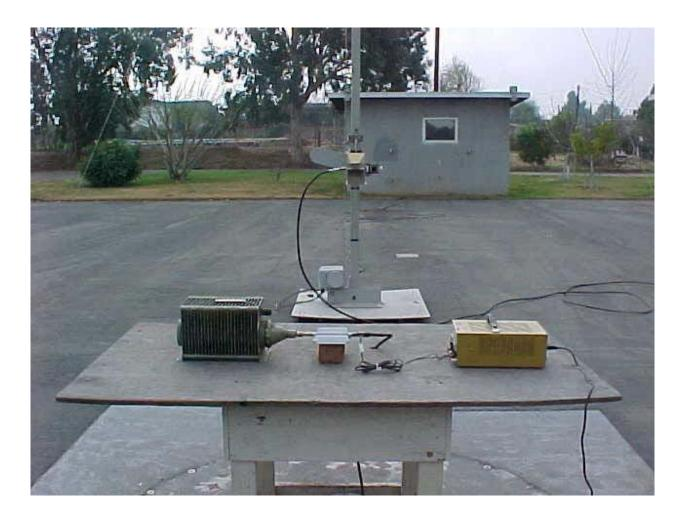
PHOTO: RF POWER OUTPUT, EMISSIONS LIMITATIONS CDMA, OCCUPIED BANDWIDTH CDMA, CONDUCTED SPURIOUS EMISSIONS AT ANTENNA TERMINALS
