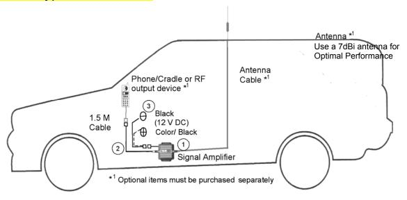
Typical Installation For Under The Seat Mounting
