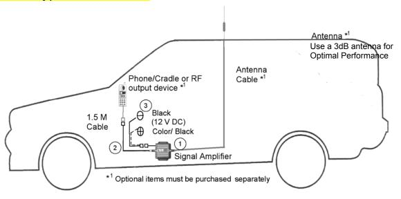
**Typical Installation For Under The Seat Mounting**
