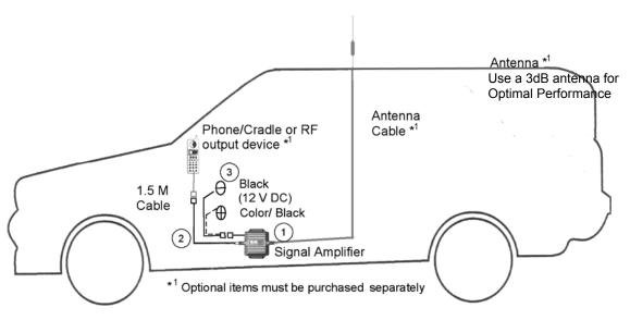
Typical Installation For Under The Seat Mounting
