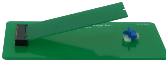
Figure 3-7: Inserting the M.2 Module into the Slot at an Angle
