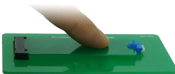
Figure 3-8: Securing the M.2 Module
