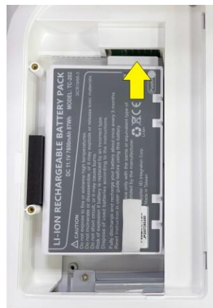
Figure 1-10: Connect the Battery Pack
