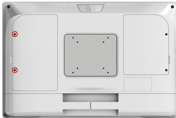
Figure 1-8: Battery Cover Retention Screws
