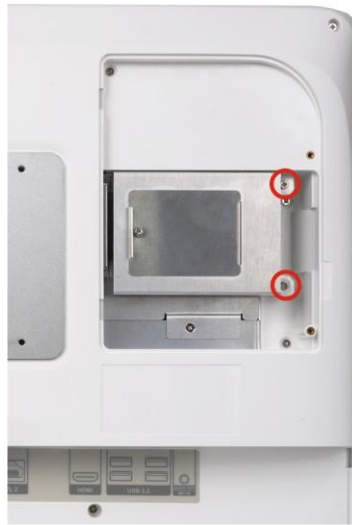
Figure 3-2: HDD Bracket Retention Screws
