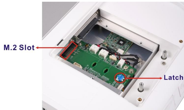
Figure 3-6: M.2 Slot Location
