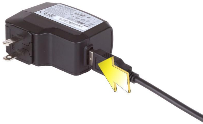
Figure 3-3: Connecting the MODAT-550A to the Power Adapter
