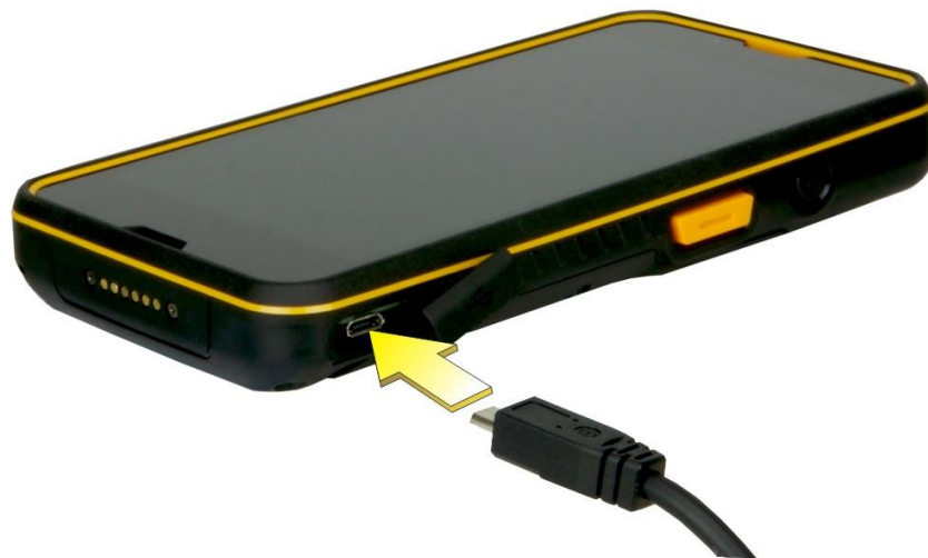
Figure 3-1: Connecting the Micro USB Cable to the MODAT-550A
