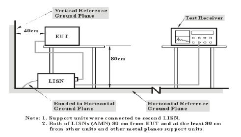
The setup of EUT is according with per ANSI C63.10-2013 measurement procedure. The specification used was with the FCC Part 15.207 limits.
