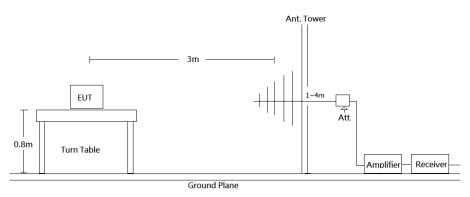
Radiated emission tests were performed in the 3 meters chamber test site, using the setup accordance with the ANSI C63.10-2013. The specification used was the FCC Part 15.209 and FCC 15.225 Limits.
