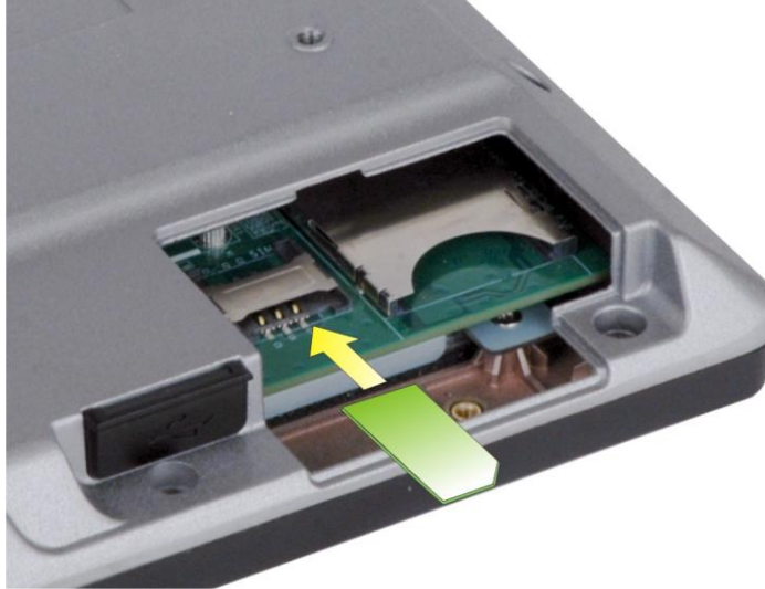
Figure 3-4: Install SIM Card
