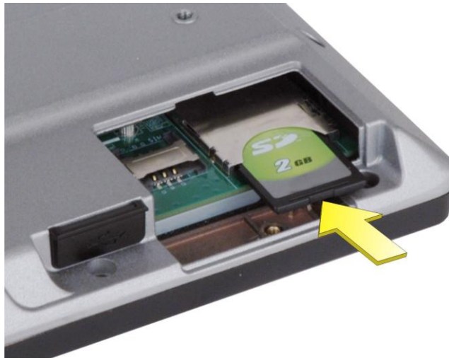
Figure 3-2: Install SD Card
