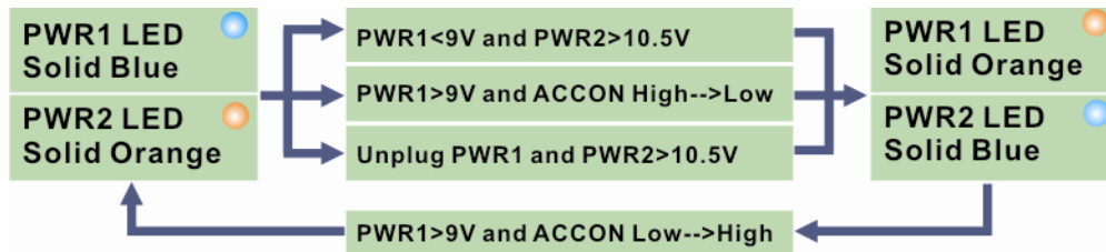
Figure 3-33: ACC On: Switch Between PWR1 and PWR2
