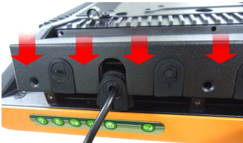
Figure 3-14: Reinstall the I/O Cover
