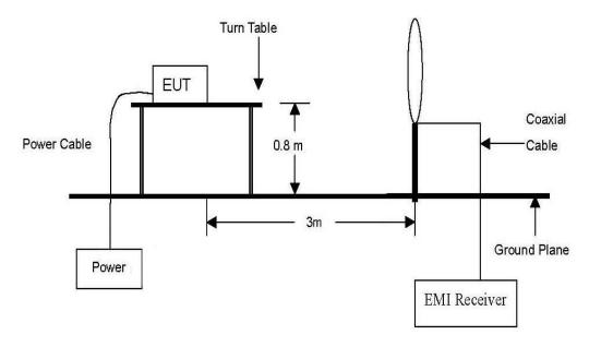
The diagram below shows the test setup that is utilized to make the measurements for emission from 30 MHz to 1 GHz Emissions.
