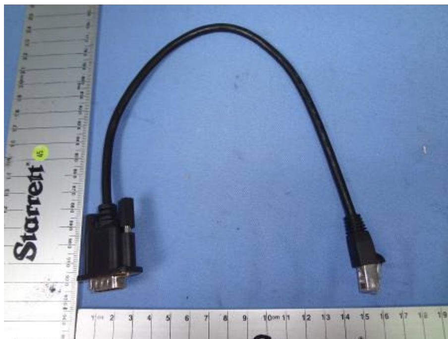
RJ-45 to DB-9 COM port cable
