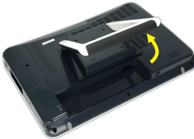
Figure 3-1: Adjusting the 2-in-1 Stand Kit
