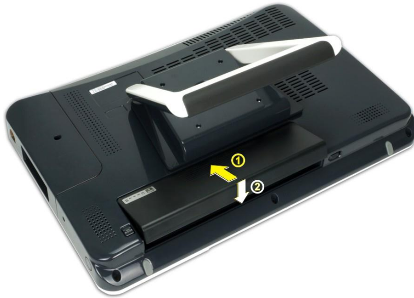
Figure 3-2: Battery Pack Installation
