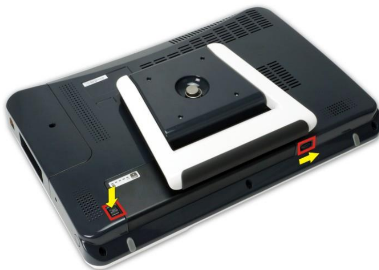
Figure 3-4: Battery Pack Removal
