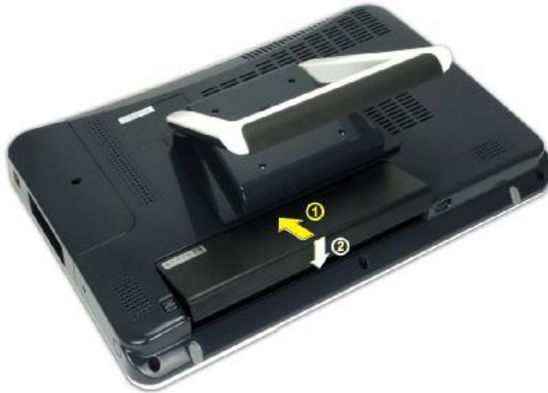
Figure 3-2: Battery Pack Installation
