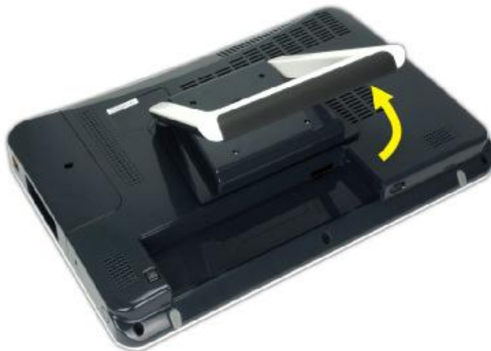
Figure 3-1: Adjusting the 2-in-1 Stand Kit
