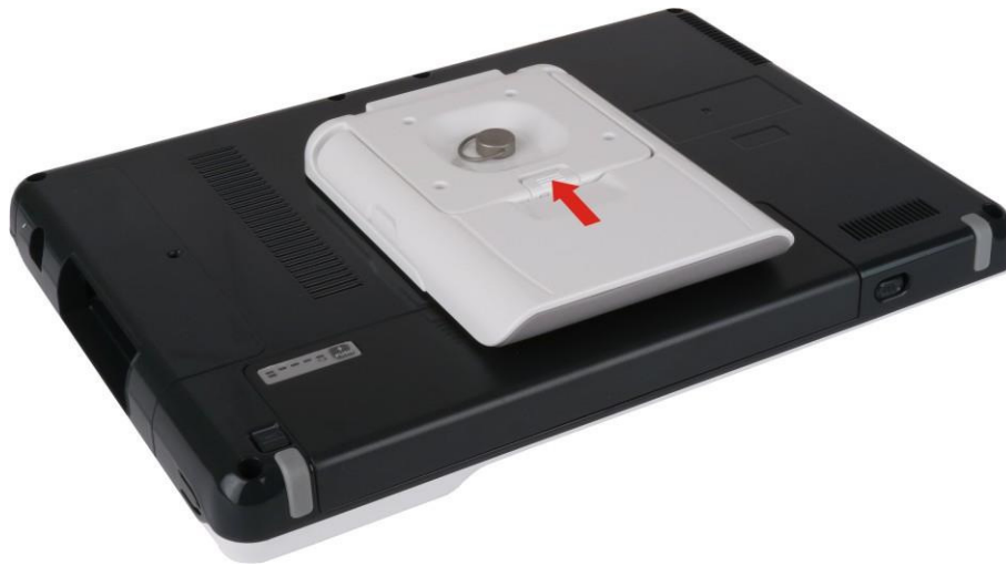
Figure 3-5: Releasing the Tablet Stand
