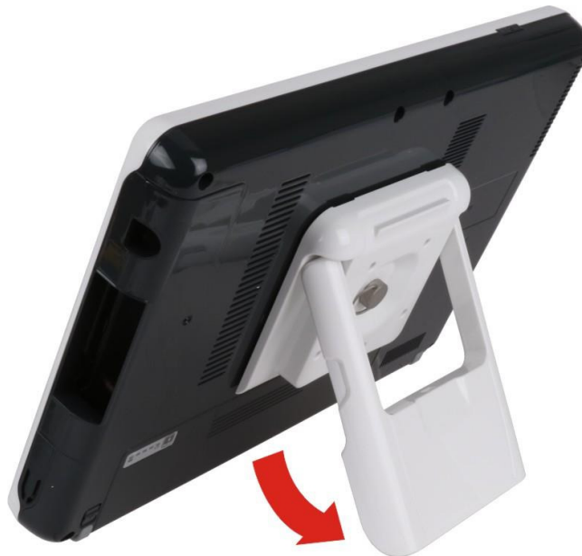
Figure 3-6: Adjusting the Tablet Stand
