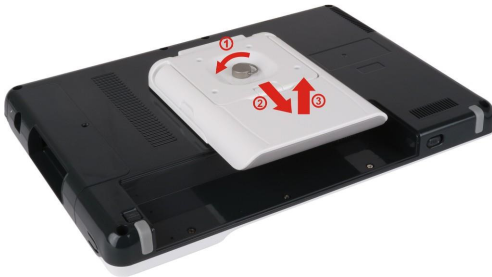
Figure 3-1: Removing the Tablet Stand Kit
