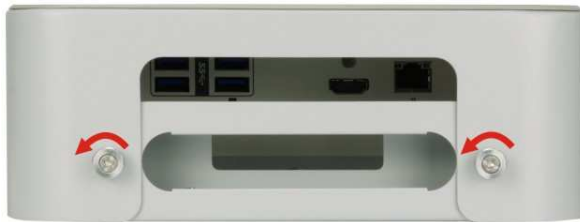
Figure 3-4: Captive Screw Removal
