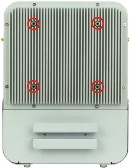
Figure 3-8: Stand Mounting Retention Screw Holes
