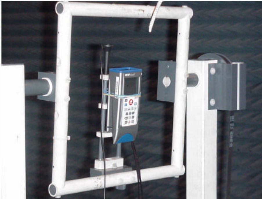
Picture 5 : Setup for the test "Spurious Radiated Emissions"
