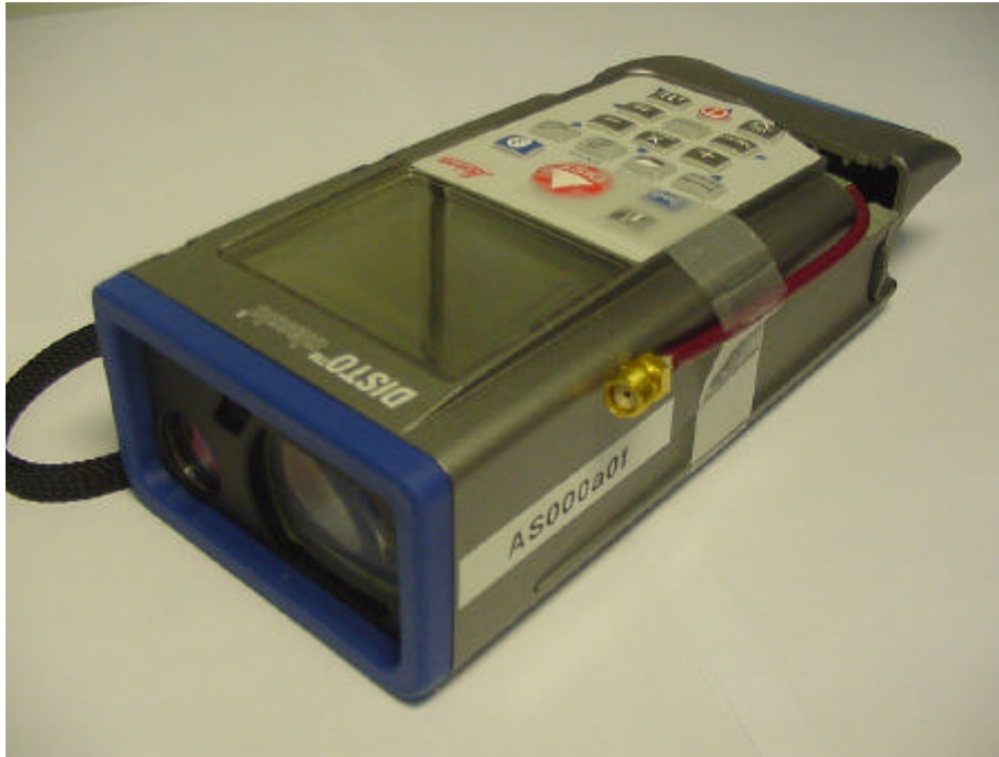
Picture 1 : EUT A (AS000a01; front, left and top side), with temporary antenna connector
