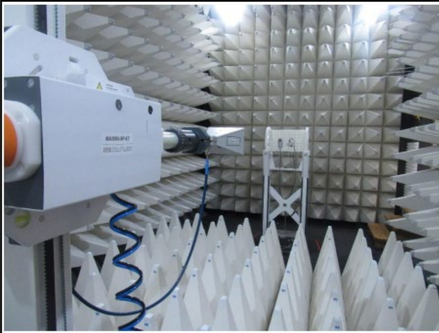
Setup for measurements above 1 GHz
