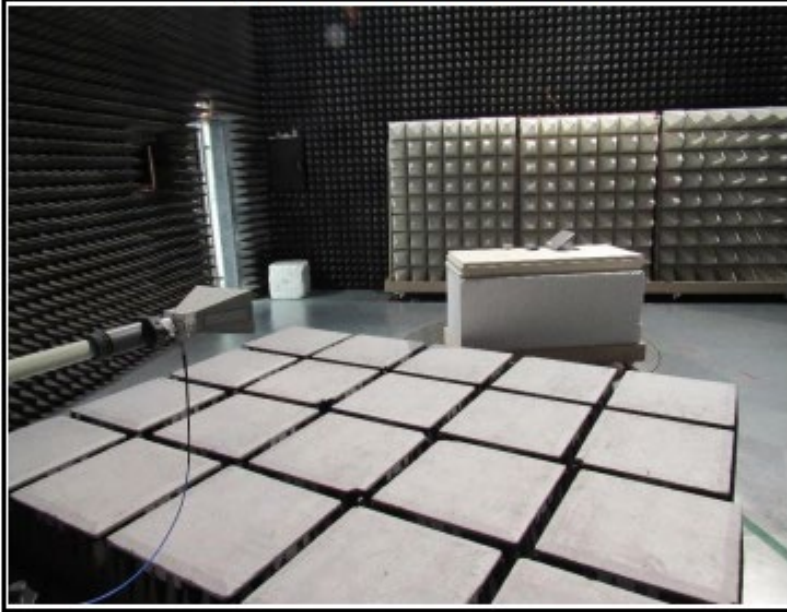
Setup for measurements above 1 GHz
