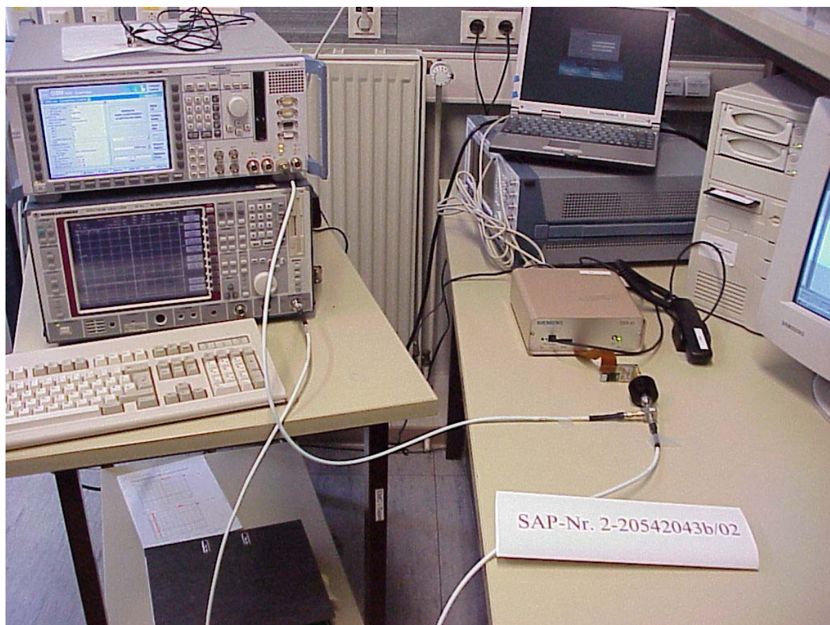
Photograph 7: Test site for conducted measurements (1)
