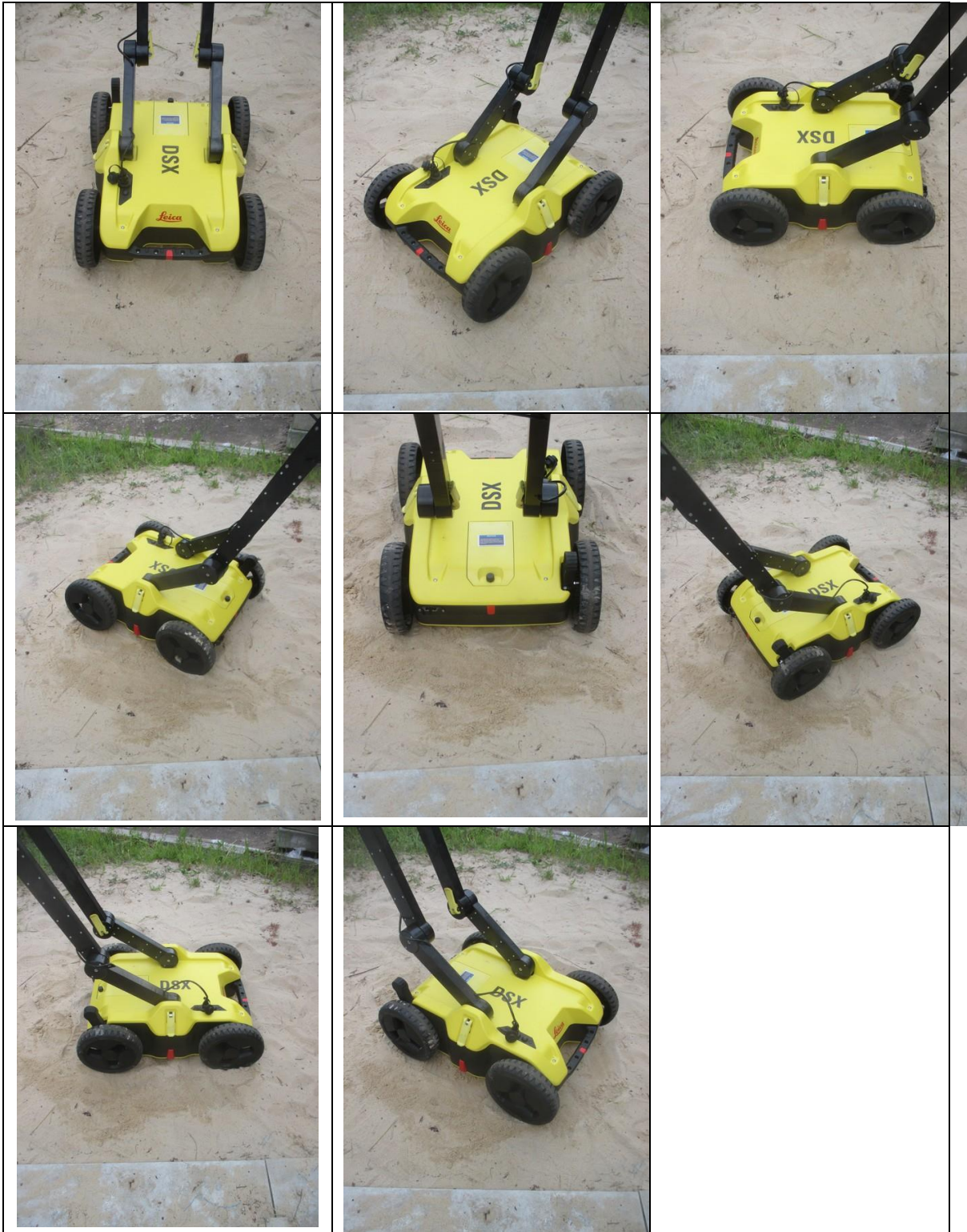
EUT Positions with 45 Degree Interval
