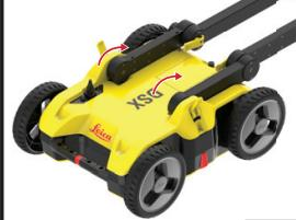
2. When the handles reach the hard-stop, lock the hinges.
