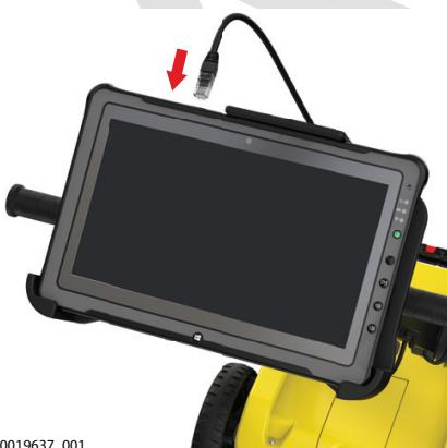
Plug in the DSX LAN cable to the tablet.
