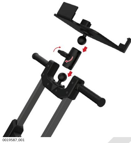
1. Mount the two RAM balls to attach the tablet to the handle:
