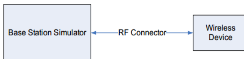
Figure 9.2 Power Measurement Setup
