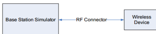
Figure 9.1 Power Measurement Setup
