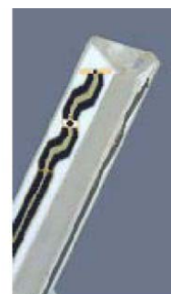
Figure 3.3 Probe Thick-Film Technique
