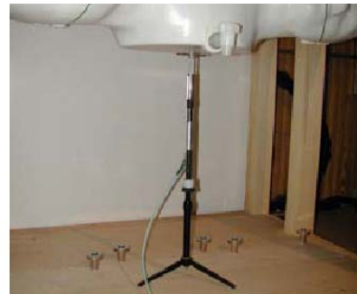
Figure 11.1 Dipole Verification Test Setup Diagram & Photo
