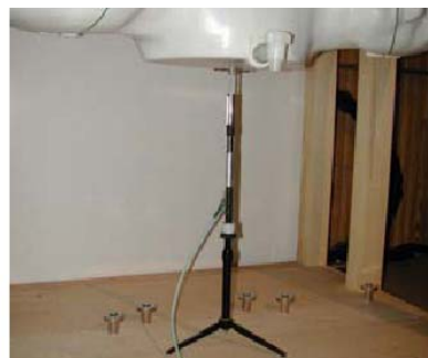
Figure 11.1 Dipole Verification Test Setup Diagram & Photo
