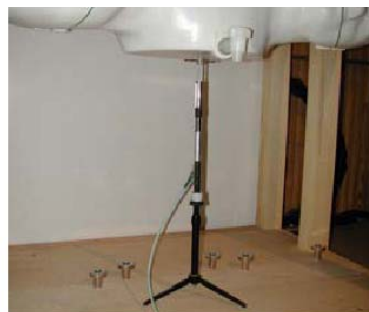
Figure 11.1 Dipole Verification Test Setup Diagram & Photo
