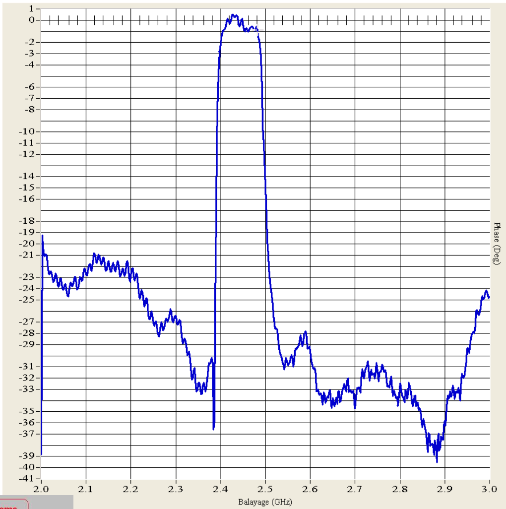
Figure 2: Typical Antenna peak gain vs Frequency
