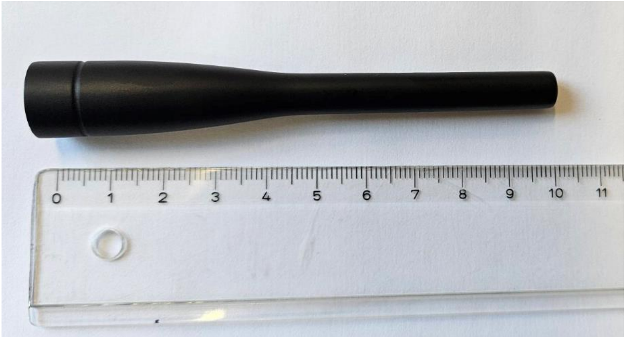
External LTE antenna
