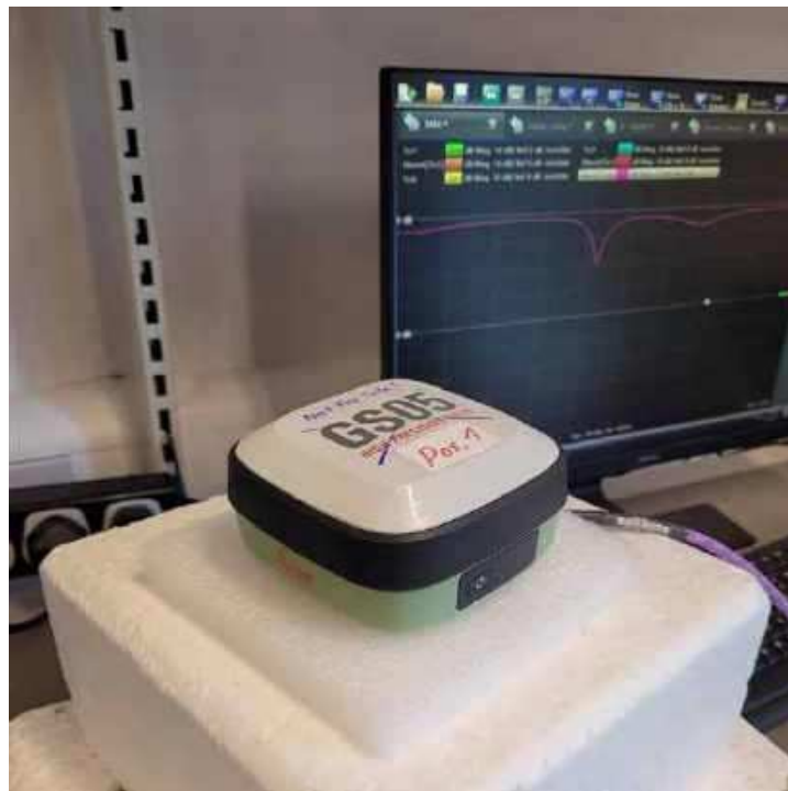
Figure 3 Test Setup for VNA Measurements
