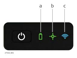
a Battery LEDb Position LEDc Connectivity LED
