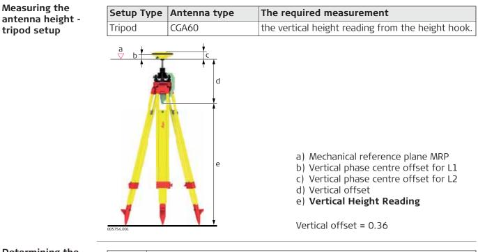
Determining the antenna height with the height hook step-by-step
