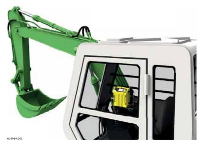
The product must not be installed on the tool of the machine and/or on mechanical components that move the tool. Tools include for example bucket of excavator, blade of dozer, screed of paver. Mechanical parts include for example boom and stick of an excavator, hydraulic cylinder of a dozer or tow arm of an asphalt paver.
