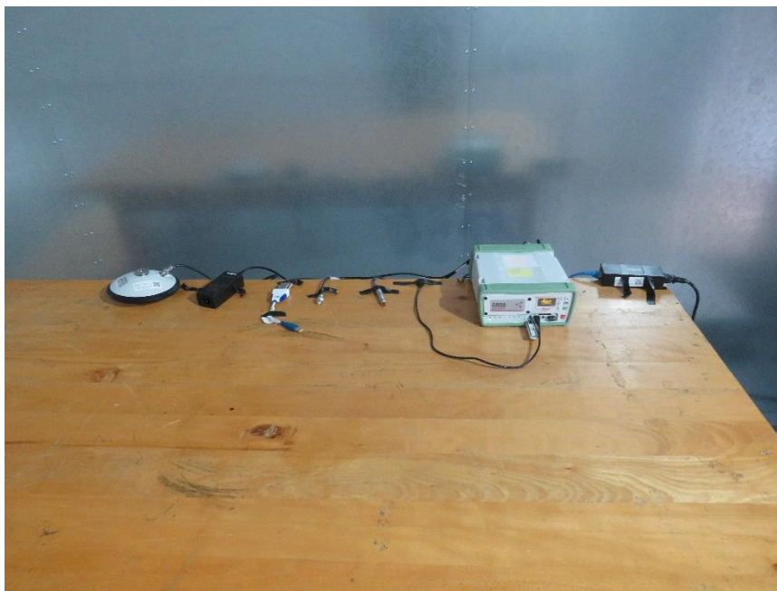
Setup for measurements 150 kHz – 30 MHz (with PoE)
