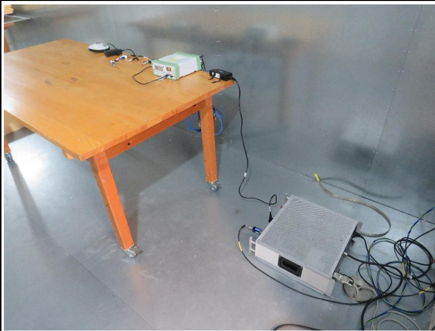
Setup for measurements 150 kHz – 30 MHz (with PoE)
