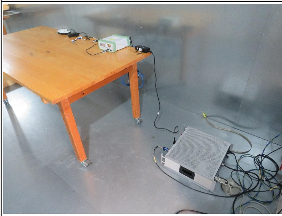
Setup for measurements 150 kHz – 30 MHz (with PoE)
