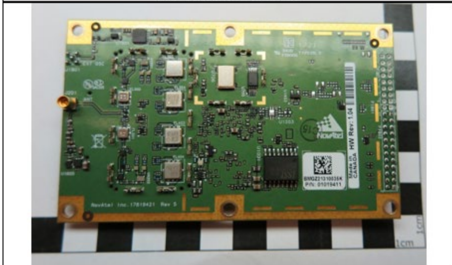
PCB 5 TOP: Detail no Shields
