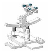
The SAR in the phantom is approximately inversely proportional to the square of the distance between the source and the liquid surface. For a source at 5 mm distance, a positioning uncertainty of  $\pm$  0.5 mm would produce a SAR uncertainty of  $\pm$  20 %. Accurate device positioning is therefore crucial for accurate and repeatable measurements. The positions in which the devices must be measured are defined by the standards.4. Tissue Simulating Liquids
