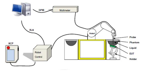
COMOSAR is a system that is able to determine the SAR distribution inside a phantom of human being according to different standards. The COMOSAR system consists of the following items:
